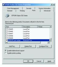
9. The installation is done. You can print a document to test it, this printer should be on the printer list already, as shown in the following window.
